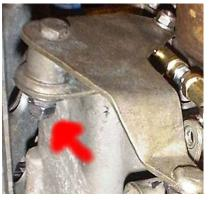
Remove the bell-crank nuts (shown left), this is a Nyloc and half nut. When removed, the bell-crank
