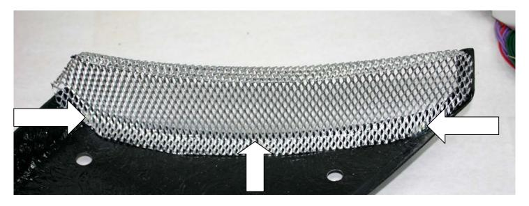
Once satisfied clean the inner carbon panel with the cleaner sachet and glue the mesh to the scoop (see picture) use a long thick bead of adhesive and smear down being careful of the mesh sharp edges.
