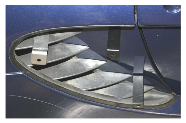
Mark the vehicles side panel through the two "U" shaped brackets in the centre hole (middle of the 5 holes).
