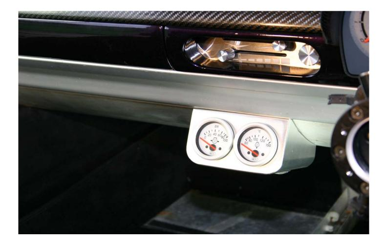
The gauge pod simply clips in place of the interior light unit and the interior light unit fits in the rectangular slot in the gauge pod. The pod is held in by the tension of the "flap" designed into the pod casing.
