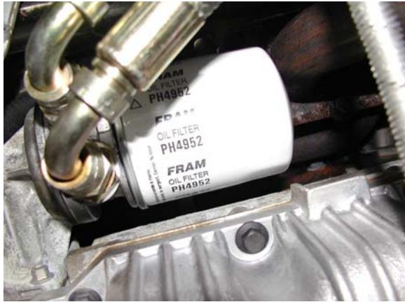
Connect the new braided hoses to the oil cooler unit as shown in top picture ,the short braided hose fits to the Right hand side of the cooler and the longer hose fits to the Left hand side.
