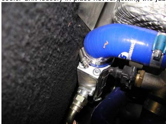
Fit the oil cooler loosely on the rear engine outlet pipe.
