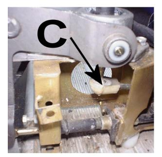
Remove lever from the base unit leaving the top half of the plastic cup in place.
