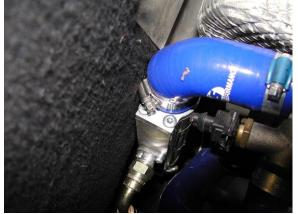
Fit the oil cooler loosely on the rear engine outlet pipe.
